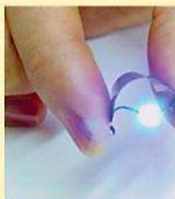
Front Edge Technology battery powers a light-emitting diode.
